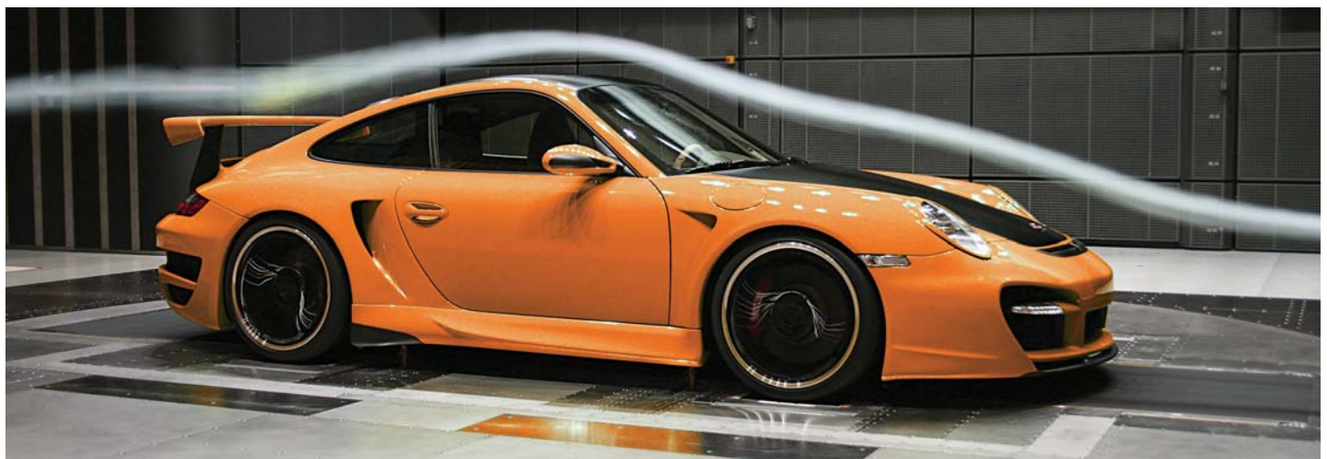
TECHART GTstreet Aerodynamikpaket in der Windkanalprüfung Wind tunnel testing of the TECHART GTstreet aerodynamic kit
